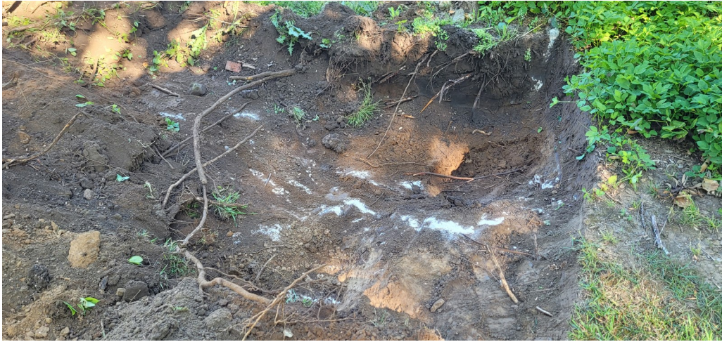
Photo 3: View of weathered, hummocky bedrock surface in TH-2.
