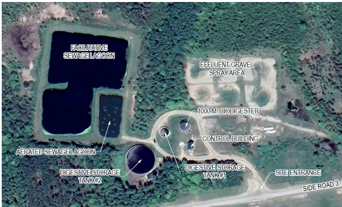
Figure 3.1 – Site Plan of the Derby WWTW with BioGrid System and Sewage Lagoons
