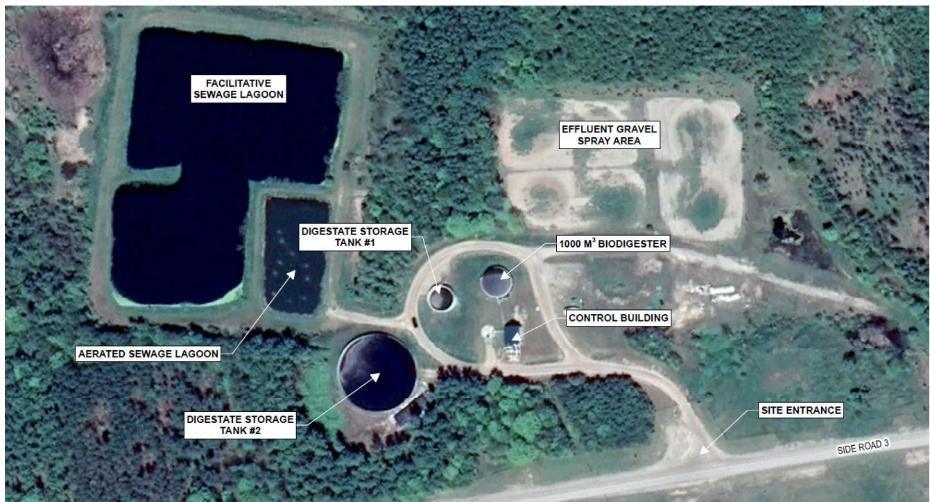
Figure 2 Site Plan of the WWTW with BioGRID System and Sewage Lagoons
